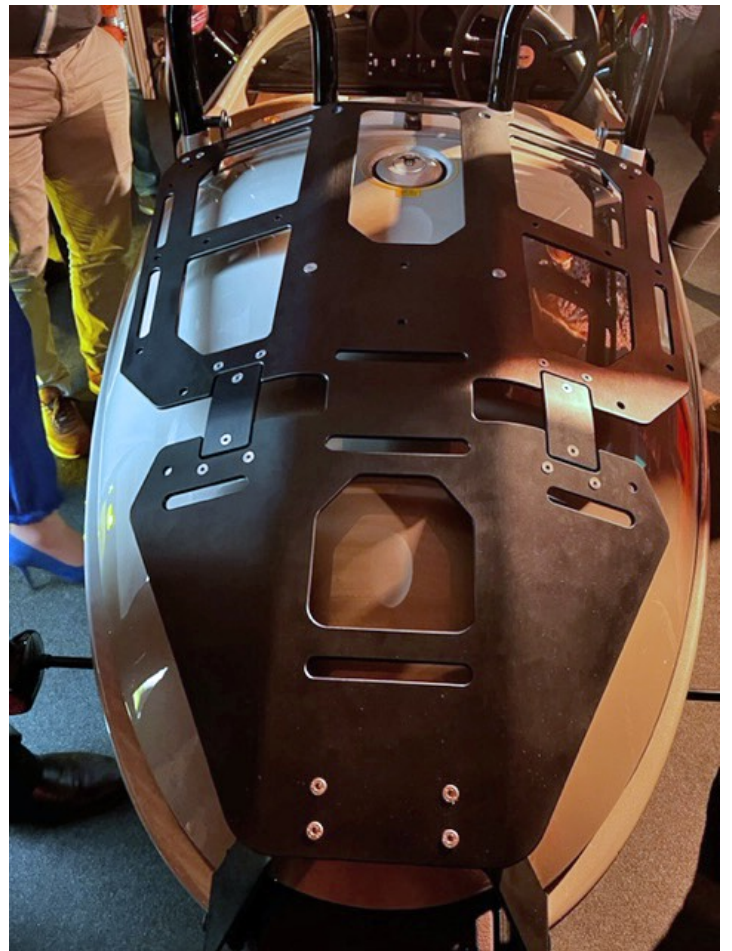
A huge removable luggage rack for carrying very large volumes of gear plus fitted soft or hard luggage on the sides
