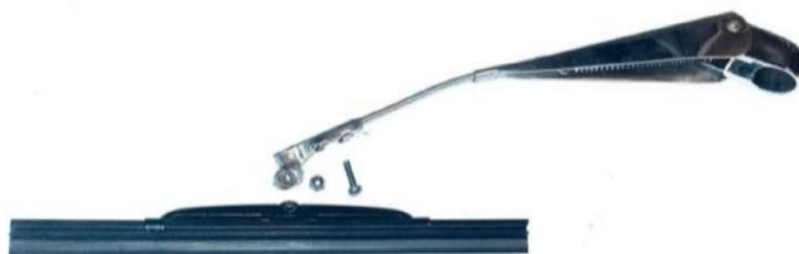
9. Now clip your new assemblies onto the waiting wiper arms on your Mog. There is a photo below of the old and new compared attached. They are resting on a sheet of paper to increase the contrast as they tend to disappear into the darkness on the windscreen. I was able to source the 2.5mm x 10mm stainless screws and locknuts on ebay without having to buy in large quantities.
