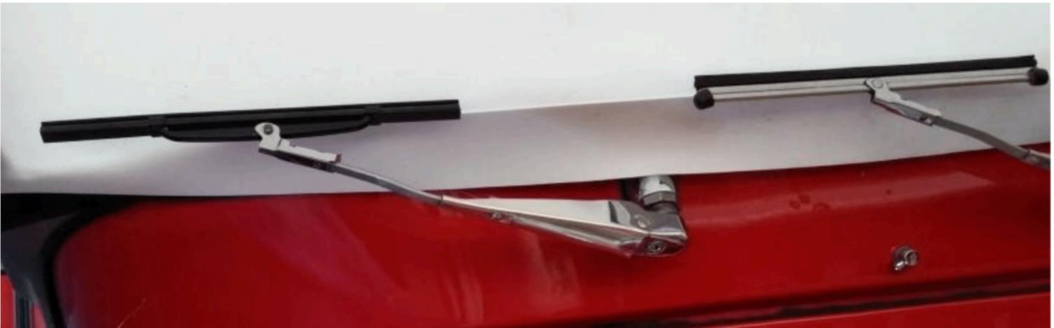
The image above shows both the original wiper alongside the improved version on the left; a sheet of white paper covers the windscreen to enhance the blade image.
