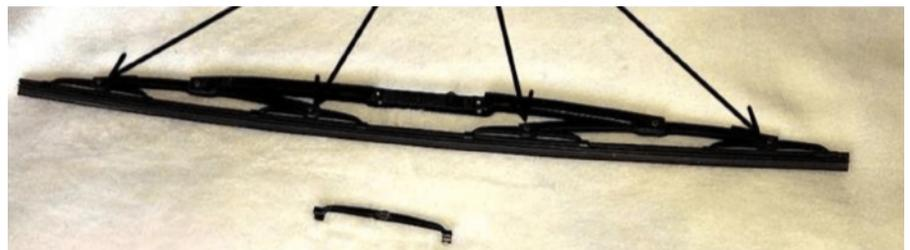
5. Remove the small pivot-rivet that attaches the blade to the arm section. Set aside the old blade and you have the clip-on part of your Mog's wiper arm that you need.
