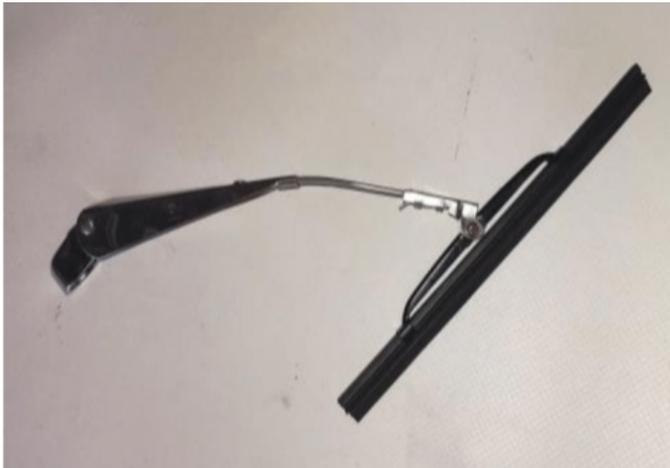
Essentially what I've done is cut down and adapted a Bosch wiper blade intended for a BMW saloon into three Mog sized blades as you can see in the picture below. Any donor blade will do as long as it has the small curved yokes in the pictures.
