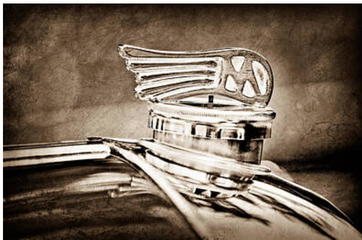
The wrong flying M is mounted - should be the flat one
