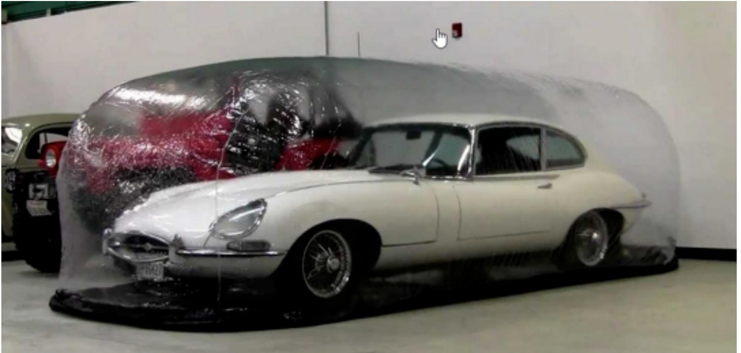
The base is a strong durable rubber, probably because you are driving the car on to it, and of course would normally sit on a concrete floor. Around the perimeter is a zipper attaching the bag section to the floor.
