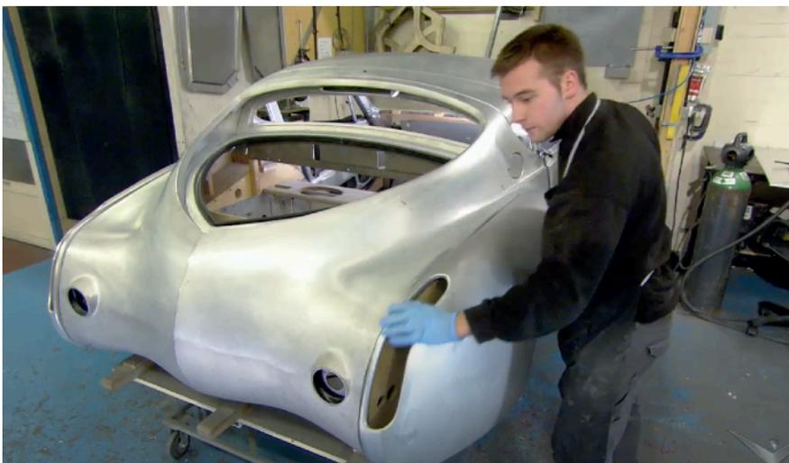
Attaching a wing from "How It's Made"
