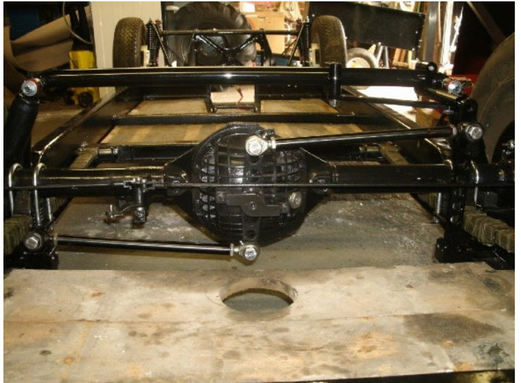
Owen's self-designed and built Watts Linkage
