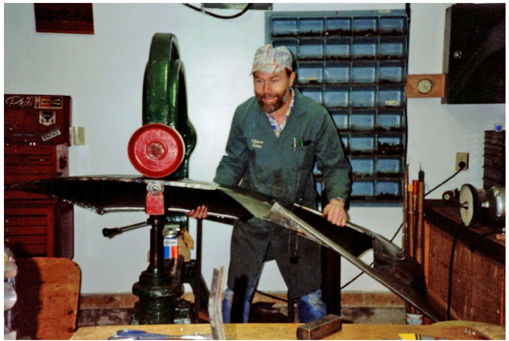
Phil shaping the panels
