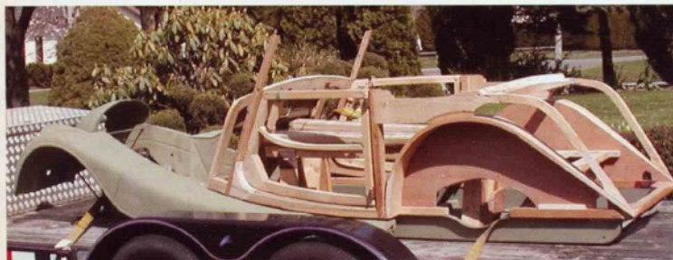
Basic wood frame test fitted to chassis
