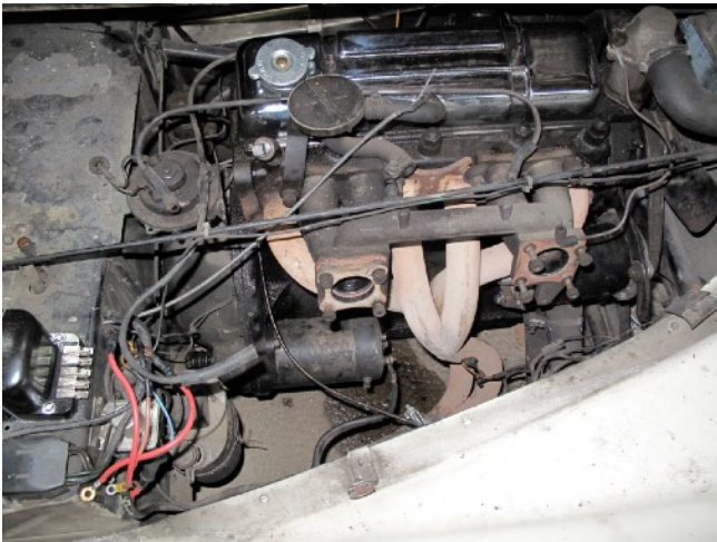
Top: Engine showing carbs and freeflow manifold Right: Vic's car after the garage fire
