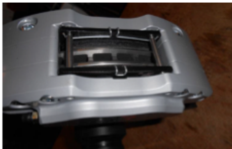
Above - how to fit the pad retaining springs.
