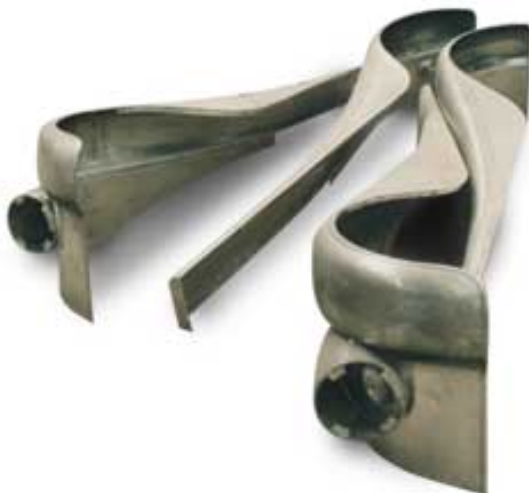
Steel and aluminium wings for a Morgan Plus 8, (Courtesy of Vintage Wing and Radiator)
