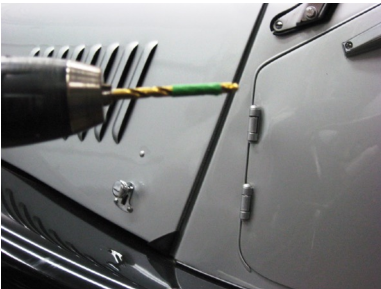
3. Drilling the door wood frame from the inside to insert the T-nut. It is important to refer to the drilling chart to use the right size drill: 7/32 inches. The T-nut should be press-fitted into the door wood frame. Put a tape on the drill to indicate the depth of the hole to be drilled.
