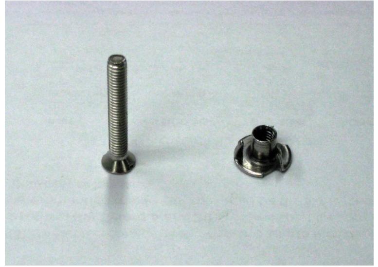
6. Top view: Stainless steel screw, size 8/32 x 1 inch 1/2 and 3 prong T-nut.
