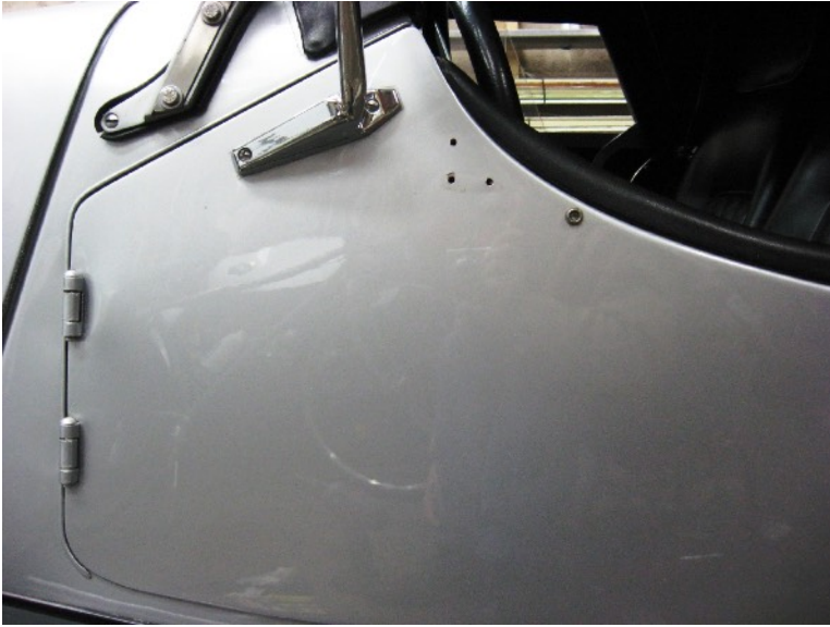
1. Unscrew the side screen knob
