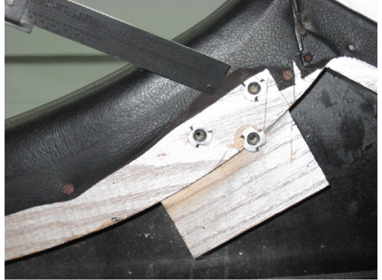
8. Door frame with the 3 T-nuts
