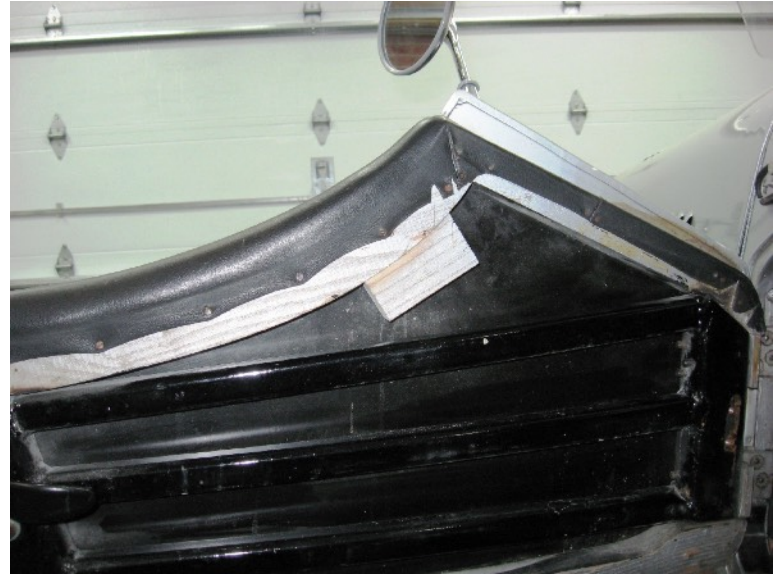
2. View inside door. Drill through the door wood frame from outside the door through the three existing door knob holes to the inside of the door. Important: Use a small drill size no more than the original size of the wood screw that needs to be replaced. These small holes will be used as a pilot when drilling for the T-nut.
