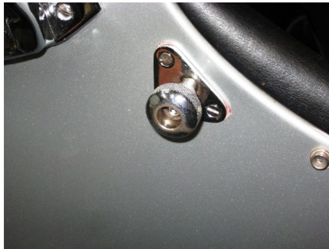
9. Side screen door knob installed with the new Stainless Steel slot screw. The result is very solid!
