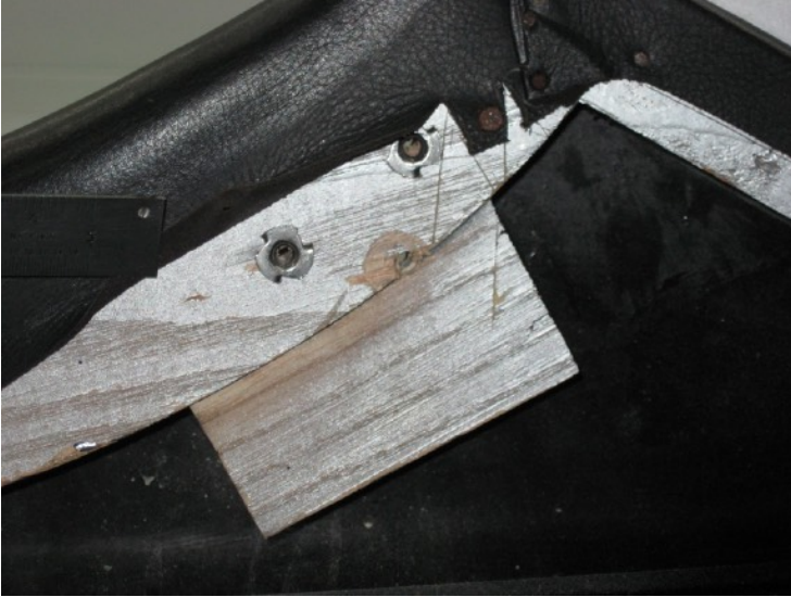
7. Door frame with 2 of the 3 T-nuts
