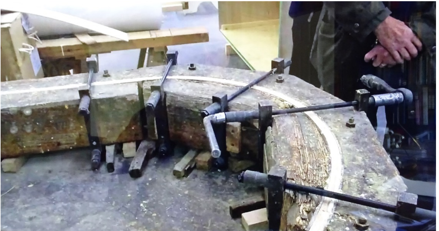
Photos courtesy of Nigel Matthews from his trip to the factory in 2012 Pictures showing the shaping of the wood for the wheel arches.
