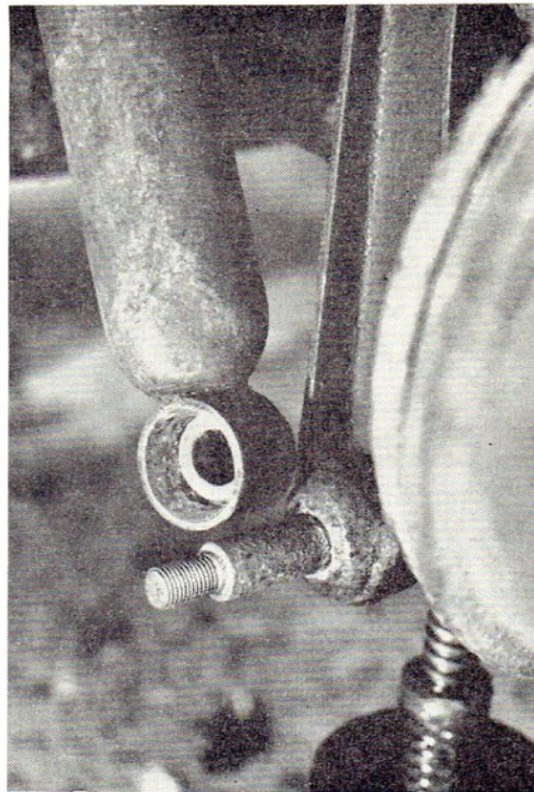
Once the nut is removed the old unit can be prised off and rubber bushes removed
