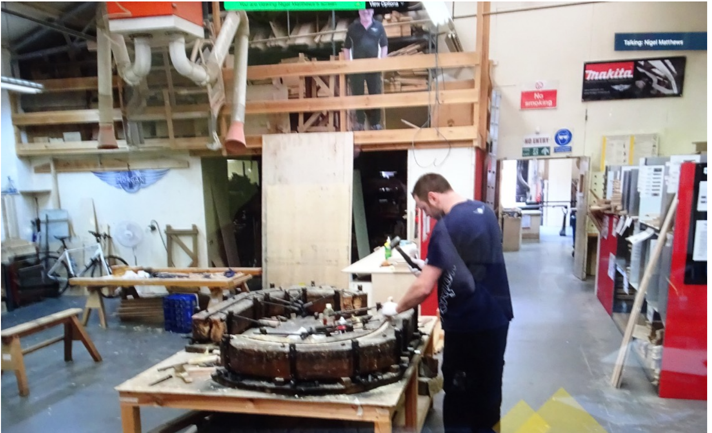
Photos courtesy of Nigel Matthews from his trip to the factory in 2012 Pictures showing the shaping of the wood for the wheel arches.
