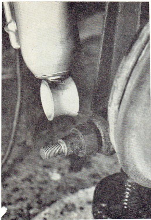
Having attached the new unit at the top end by fitting the rubber bushes first deal likewise at the lower end
