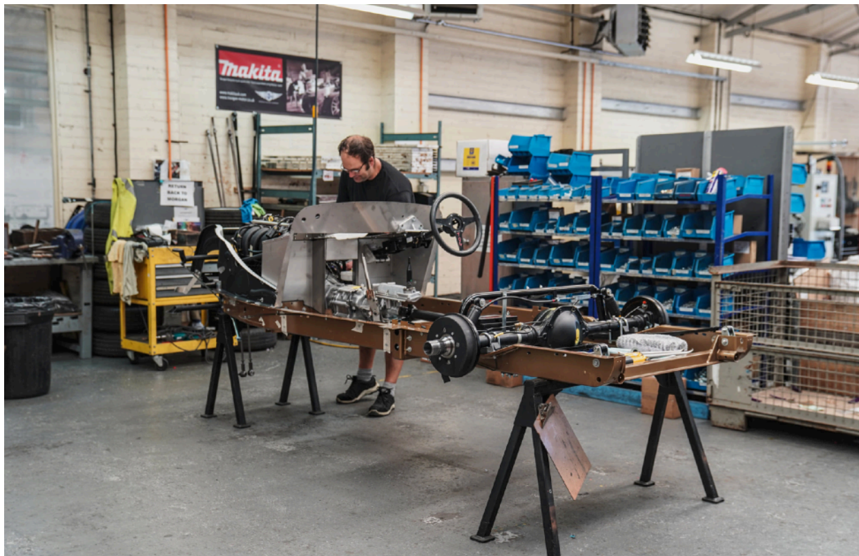
Above - The last steel chassis in the Chassis Shop at Pickersleigh Road. Below - New meets old. CX-Generation aluminum platform and the steel chassis.
