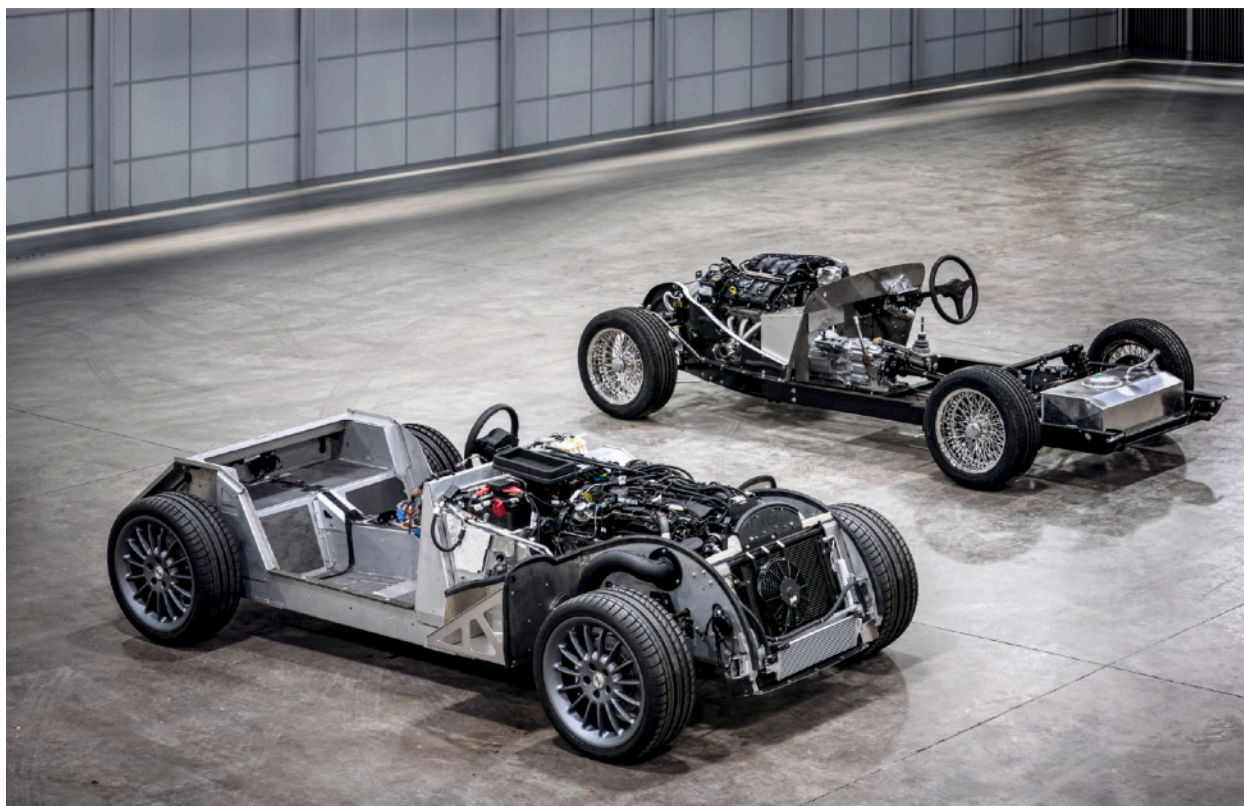
Above - The last steel chassis in the Chassis Shop at Pickersleigh Road. Below - New meets old. CX-Generation aluminum platform and the steel chassis.
